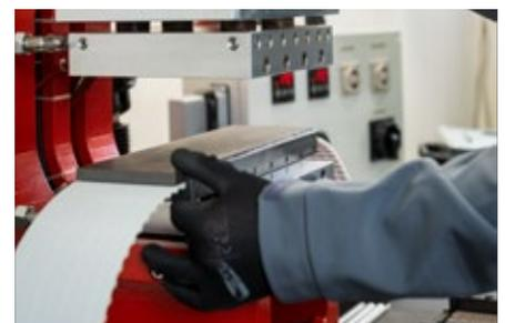
The high level of automation of the M.E.C.® Splicing, in both the welding and the cooling stages, allows numerous consecutive joints to be made without the continuous presence of the operator, who in the meantime, can perform other tasks, thus saving time and costs.
